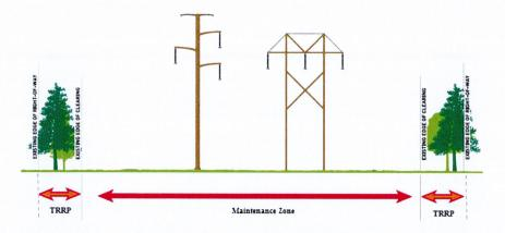
The diagram illustrates a typical right of way condition. This work is occurring within the existing edge of clearing. Your neighborhood may have a different configuration of transmission structures.
